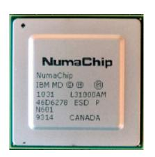
access and share all memory and I/O. The combined system runs a single instance of a standard operating system like Linux. At the heart of NumaConnect is NumaChip – a single chip that combines the cache coherent shared memory control logic with an onchip 7-way switch. This eliminates the need for a separate, central switch and enables linear capacity and cost scaling in 2D or 3D Torus topologies.
